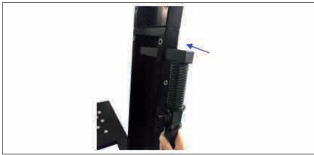
Step 13: Secure the top end of the foot pedal bar to support bracket using (4) 5/16" x 1-3/4" hex bolts, (8) 5/16" x 18 x 2 flat washers and (4) 5/16" hex nuts. Make sure the foot pedal bar is pushed all the way to the end of the support bracket (indicated by yellow arrows). Follow the same steps for the opposite side.
