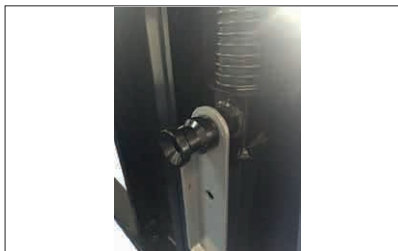
Step 15: Secure the topping to the nut on the foot pedal bar. Follow this step on the opposite side.
