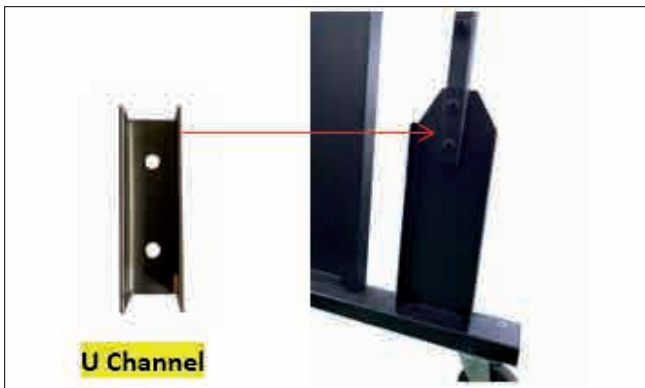
Step 14: Secure the base of the foot pedal bar to the triangular support plate by holding the lower support plate vertically up against the foot pedal bar and secure the U channel onto the foot pedal bar using (2) 5/16"x1-3/4" hex bolts, (4) 5/16" x 18 x 2 flat washers and (2) 5/16" hex nuts from the inside out. Follow the same steps for the opposite side.
